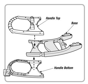
• Fit the handle top and bottom to the end of the base, as shown.
